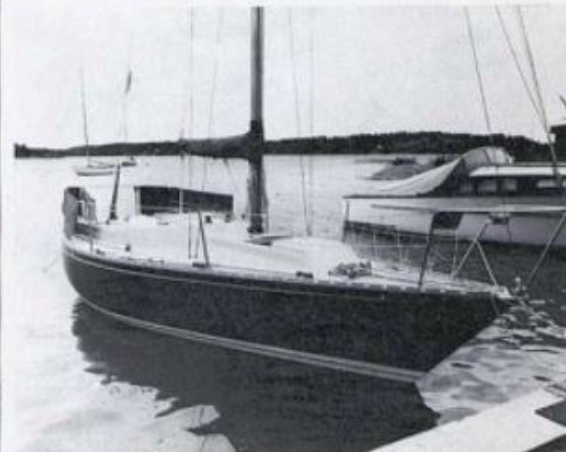
The superstructure of Blue Bird is as low as in bigger open sea racers, and because of this the interior is pretty low. The fittings seen in the photo all belong to the standard equipment.
