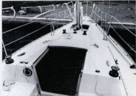
The deck of Blue Bird is clear-cut and spacious according to the character of a racer. The cabin is pretty low, but joined in the a strange, angular way. The stays are attached almost in the same point, they are easy to pass and they don't disturb the fairlead of the genoa.
