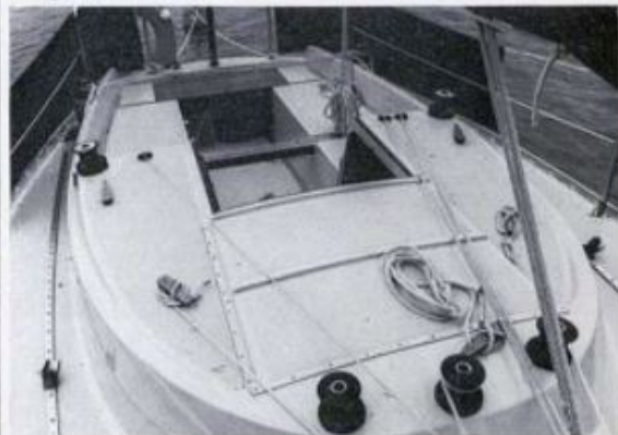
All winches of the lifters are on deck, so the mast is free of these lumps. The cockpit has good room for even four, in front of the fairlead of the mainsail two men can well work.
